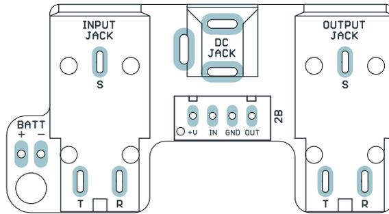
Get the two input/output jacks, the DC jack and the wire header and snap them in place on the PCB. The board is designed for them to fit securely, so you may have to press down hard to get them to snap in.
