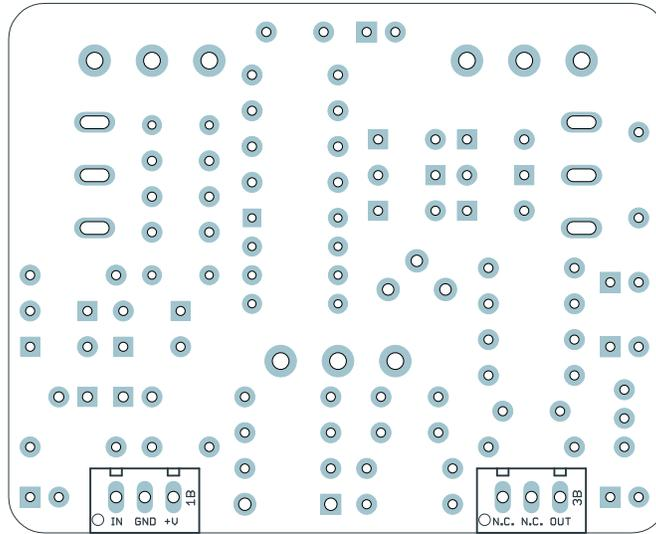
Install the two 3-pin headers (wire connectors) on the main PCB as shown above. These have a polarity pin, so as long as they are pressed all the way down, there's only one possible way to install them. They do fit pretty tightly in the holes, though, so press firmly.
