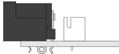
After you've soldered everything, make sure to **snip the leads on the I/O jacks as close as possible to the PCB**. There's not a lot of clearance between the bottom of this board and the top of the main PCB once everything is in place, and you don't want the pins to short against anything on accident.
